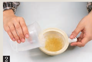
2 Pour water (Cow Hide Glue : Water =1:10) and leave overnight. Put in the refrigerator in summer. *If you have no time, you don't need leave overnight.
