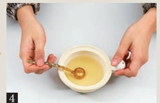
4 Complete when completely melted. Stir it well. use it after warming when harden at low temperature. *Cow Hide Glue is industrial gelatin so very pure and less contamination. Lost adhesive strength easily to add more than two times water.
