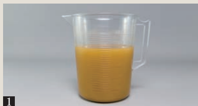
1 Add 100cc water which contains 4 grams of alum into 2000cc of the waste liquid. Stir well. Start to be flocculated gradually. (PH4.3~4.8)
