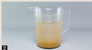
2 Add 100cc water which contains 2 grams of slaked lime into Waste liquid added alum solution. Stir well and a neutralizing reaction can be promoted. Starting to be condense precipitation. (PH6.8~8.0)
